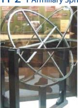
The armillary sphere is an instrument invented in China and used to measure the position of celestial bodies. During the Edo Period, this type of instrument was made even in Sendai clan, and the Japanese observed the starry sky with keen interest. There are only about 40 armillary spheres remaining in Japan, but this is the only one that is actually used to make observations. Other armillary spheres were used as models of the sky.
